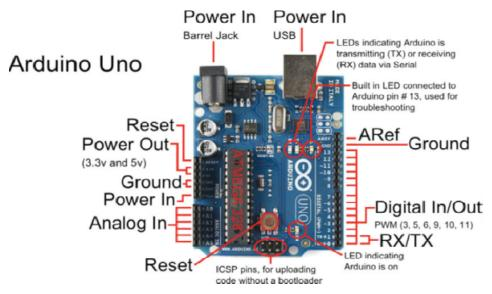
Figure 2 The pin configurations of arduino uno board
