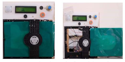
Figure 8 Hardware demonstration of automatic door opening
