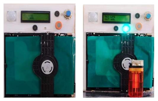
Figure 9 Hardware demonstration of liquid petroleum gas detecting system
