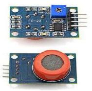
Figure 4 The photograph of MQ3 gas sensor
