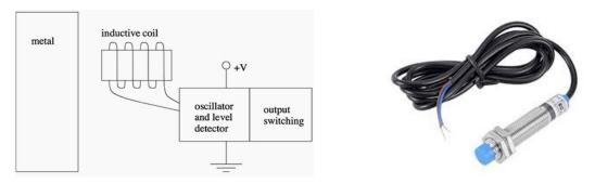
Figure 5 The photograph of inductive detector
